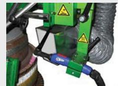
HSPS System (High Security Protection System): complete isolation of the welding area generating higher operatorsafety
