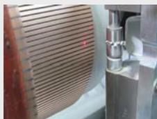
Armature rotation CNC controlled by means of a step motor with adjustable speed.
