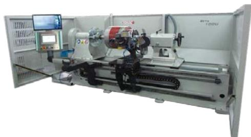
The armature is supported on rollers
